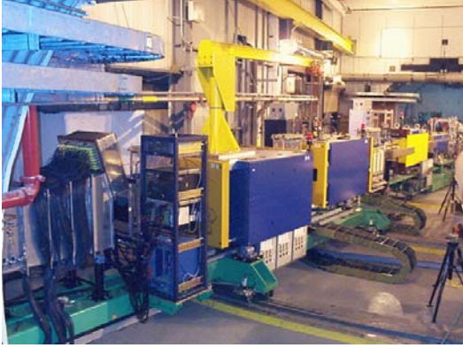
Figure 3. The Forward Spectrometer photographed from the far end towards the interaction region. The blue yokes of D3 and D4 appear in the middle of the picture. The rails for the high momentum configuration's movable platform can be seen. The RICH detector is to the left in the picture, while at the right side the yellow yoke of D2 is visible.
