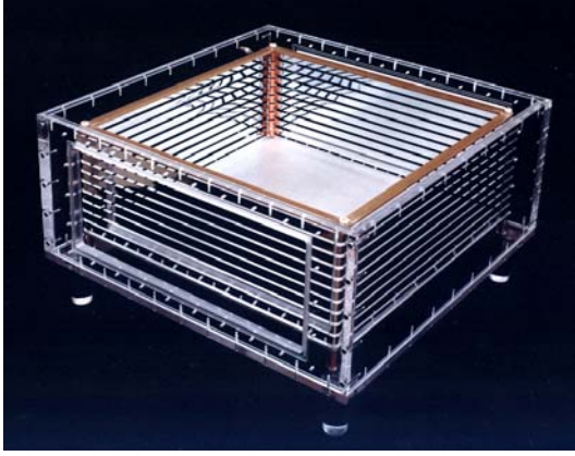
Figure 8. TPM1 Lucite box and field cage during construction.
