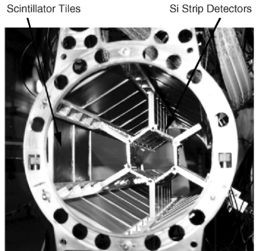
Fig. 20. Multiplicity Array with the Si strip and the scintillator tiles detectors. The beam pipe is not seen.
