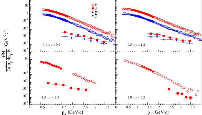
FIG. 3. (color online). (anti-)proton and (anti-)deuteron  $p_T$  spectra at various rapidities for the top 20% most central Au+Au collisions. The filled symbol part of the spectra show the  $p_T$  intervals used in the coalescence analysis. Note the limits for the deuteron range are exactly twice those used for the protons. The errors are statistical only. The horizontal bars represent the bin width.
