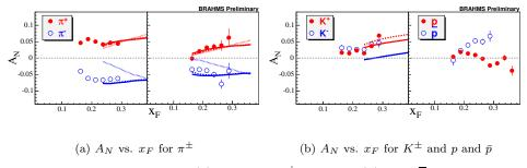
Figure 2:  $A_N$  vs.  $x_F$  for pions (a) and for  $K^{\pm}$ ,p and  $\bar{p}$  (b) at  $\sqrt{s} = 200$  GeV. Pions are measured using FS at 2.3° (left panel) and 4° (right panel), and kaons and protons are measured at 2.3°. The curves are from the twist-3 calculations with (line) and without (broken) sea- and anti-quark contribution. Prediction from Sivers effect is shown with dotted lines. Errors are statistical only.
