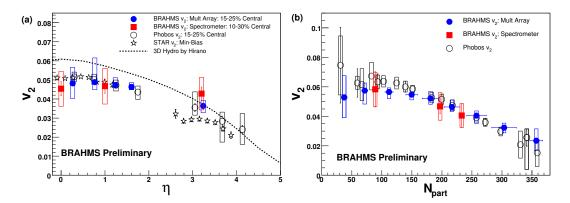
**FIGURE 1.** (a) Integrated  $v_2$  versus  $\eta$  for charged hadrons. The BRAHMS spectrometer results are consistent, but systemmatic errors with the spectra may distort the shape. For comparison, a 3D hydro model results [11] are plotted. (b) Integrated  $v_2$  versus  $N_{Part}$  for charged hadrons within  $-1.0 < \eta < 1.0$ .
